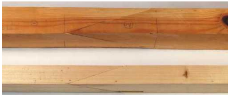
▲ Pic.8 Two practice scarf or bird's mouth joints useful for sawing practice
